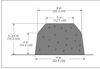
Figure 5. Cross sectional view of static obstacle for traction tests
