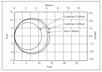
Figure 4. Clearance circles for turf work trucks
