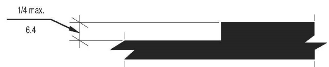
Fig. 303.2 Vertical Changes in Level
