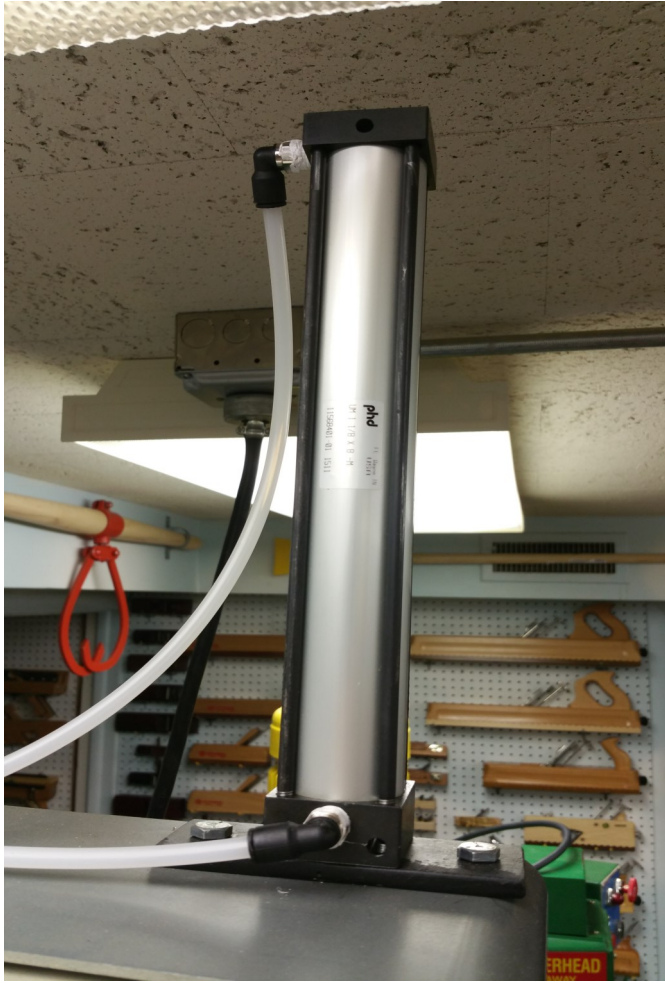
Fig. 9: Two-Way Pneumatic Cylinder
