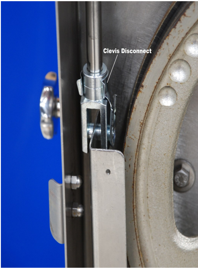
Fig. 6: Quick Disconnect Clevis
