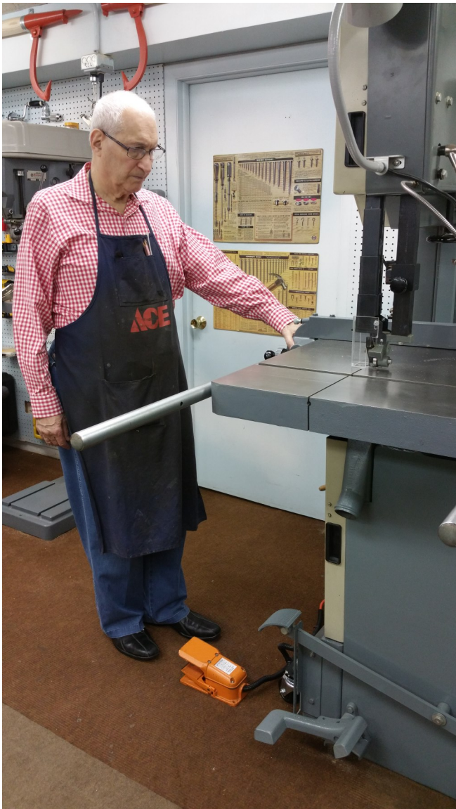
Fig. 14: Fully Guarded Band Saw Blade, Pedal is not Depressed
