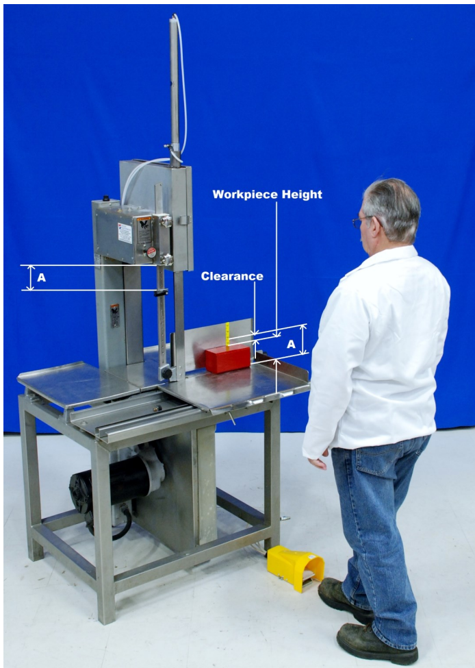
Fig. 2: Retrofit Meat Saw With Foot Pedal Released—Workpiece height plus clearance = A; Clamp setting = A; Guard touches table top
