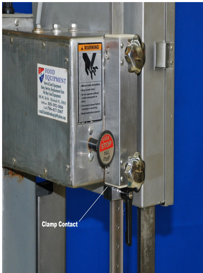
Fig. 4: Retrofit Controls: Push Stop/Pull Start, Two Friction Knobs, Clamp
