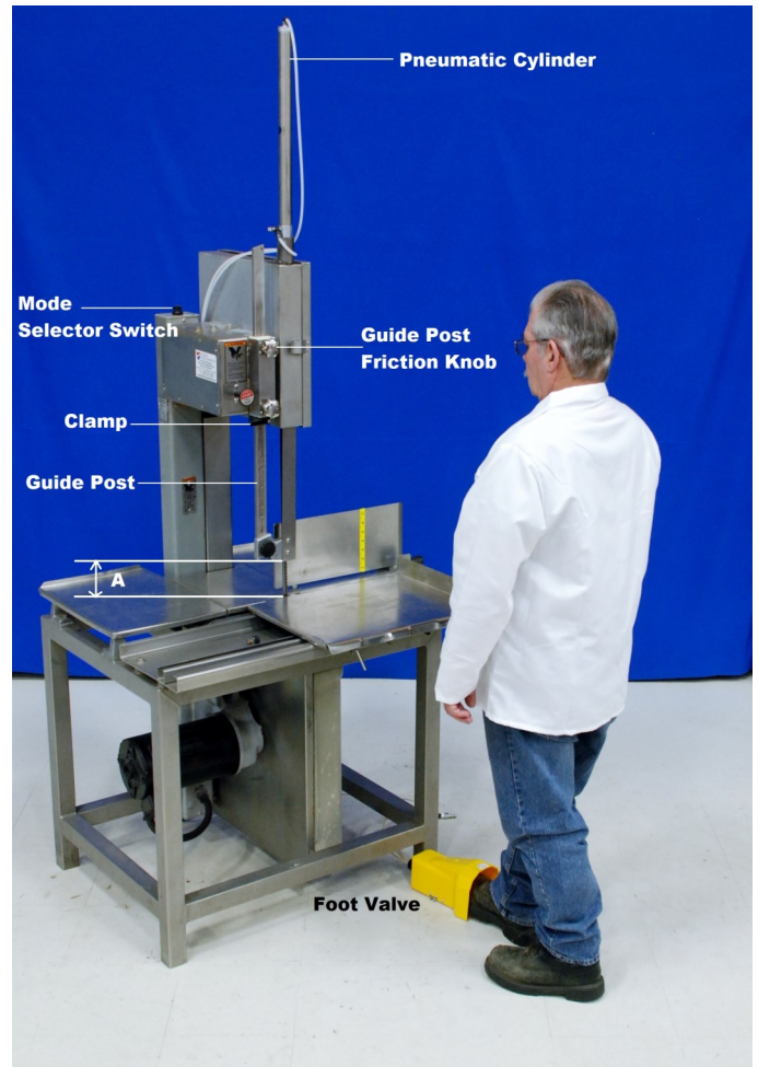
Fig. 3: Retrofit Meat Saw with Depressed Foot Pedal—Pneumatic cylinder exposes blade height = A
