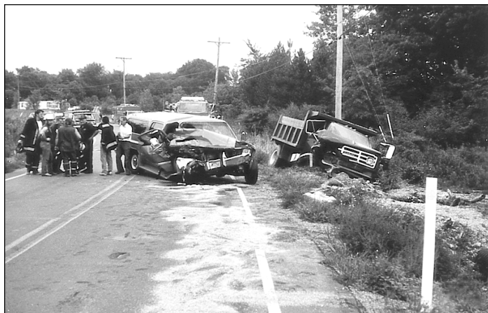
Fatal accident caused by loss of kingpin from truck steering system
