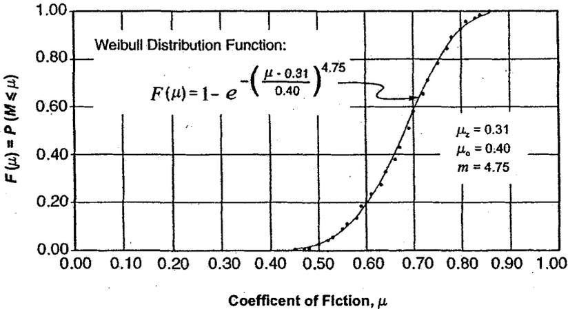
Figure 4. Cumulative distribution function: Coefficients of friction.
