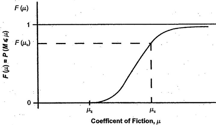
Figure 2. Cumulative distribution function: Coefficient of friction.
