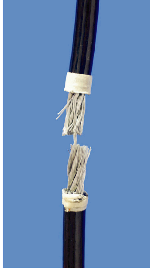
Figure 3b - Right Cable Reduced to 6 Wires
