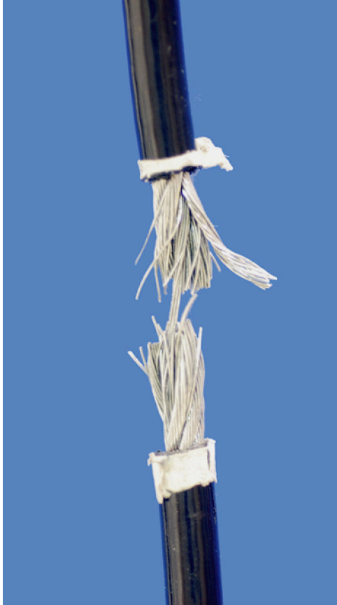
Figure 3a - Left Cable Reduced to 6 Wires
