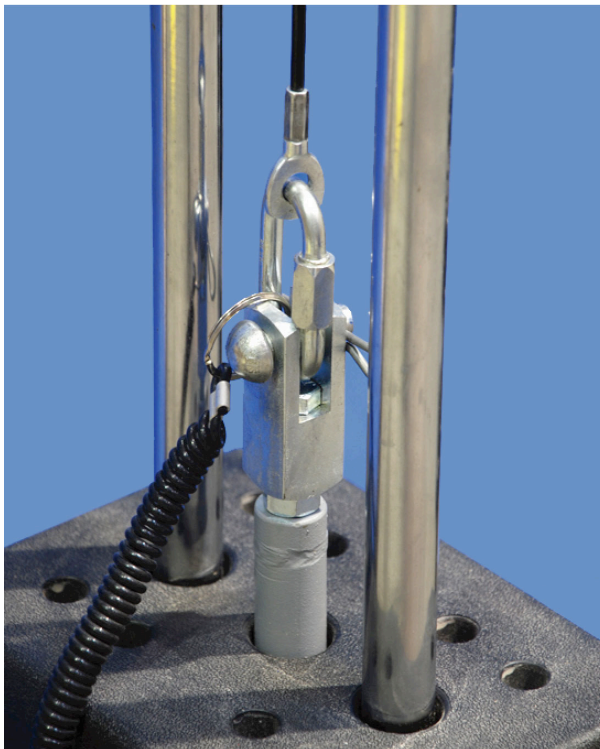
Figure 1d - Lower Termination
