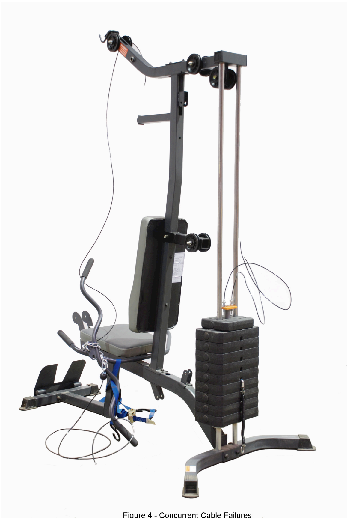
Figure 4 - Concurrent Cable Failures
