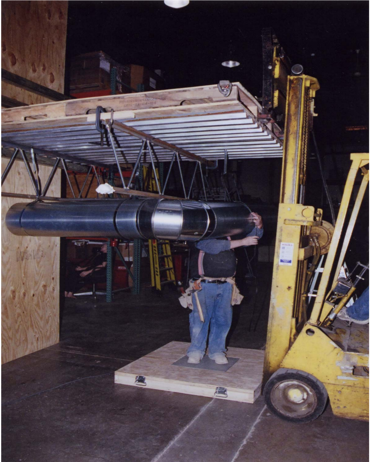
Photograph 1: Candidate HVAC Workman Supported by Force-Plate
