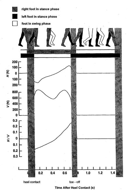
Figure 1. Contact forces during straight walking (after Grönqvist, Rolne, Jarvinen, & Korhonen, 1989). Notes. Gait phases in normal level walking with typical horizontal force (H), vertical force (V), and their ratio (H/V) for one step (right foot). Critical from the viewpoint of slipping are the heel contact (especially peaks 3 and 4) and toe-off (peaks 5 and 6). N—Newtons.
