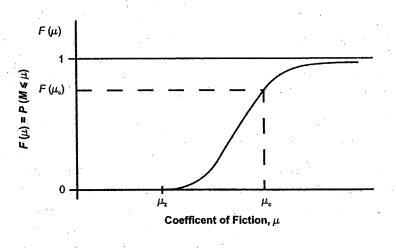
Figure 2. Cumulative distribution function: Coefficient of friction.
