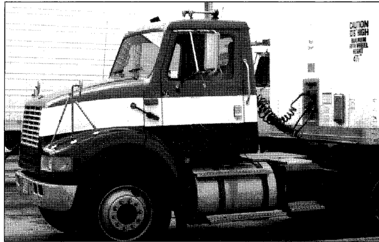
Figure 1 - Semi-Trailer with Coiled Brake Air Hoses
