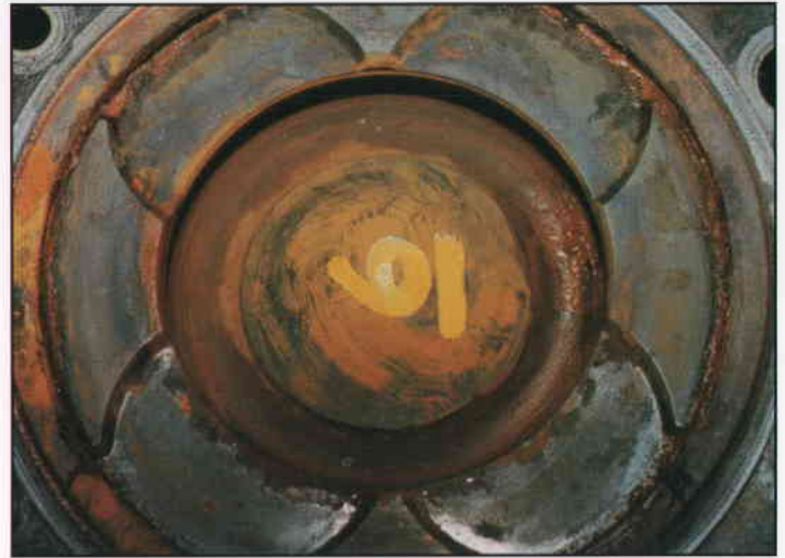
Photo 6 - Piston Valve Contact (South Engine)
