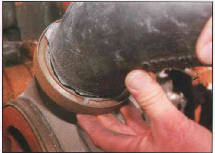
Photo 11b - Turbocharger Outlet Elbow (South Engine) Mechanical Failure
