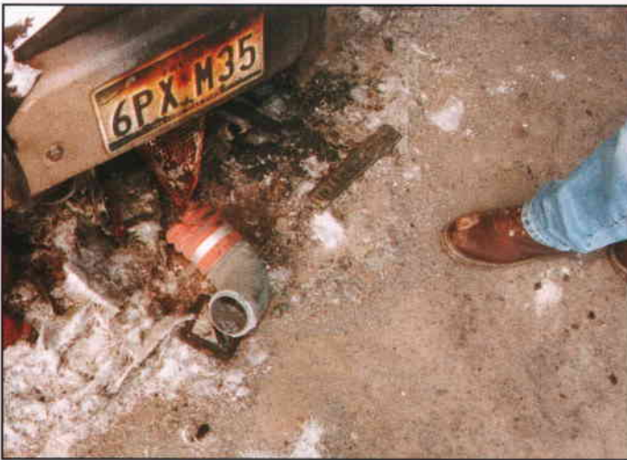
Photo 10 - Turbocharger Outlet Elbow (South Engine)
