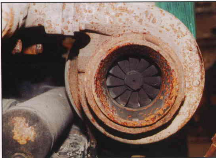
Photo 2 - Turbocharger Impeller (North Engine) Soot Covered
