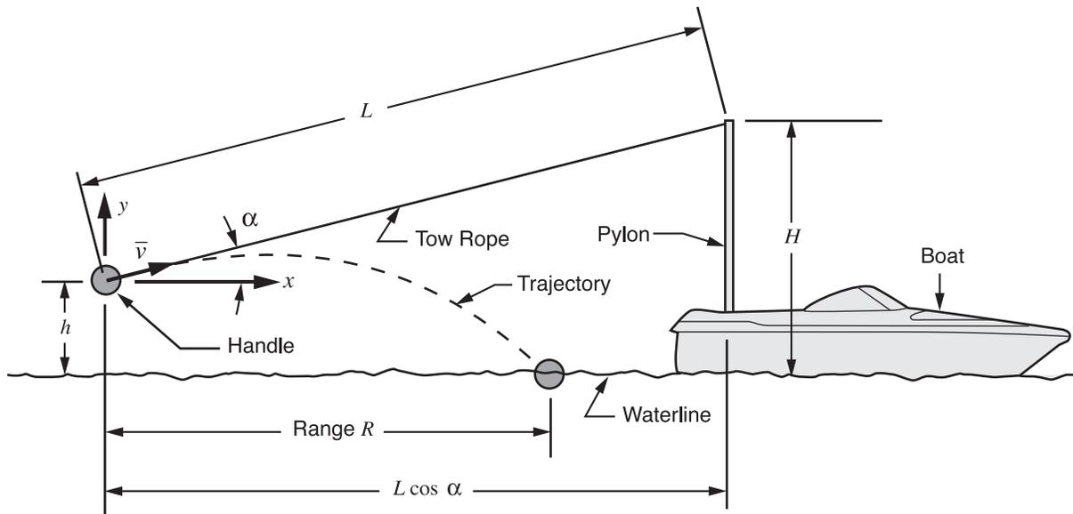
Figure 2. Wakeboard System Geometry: Handle Trajectory
