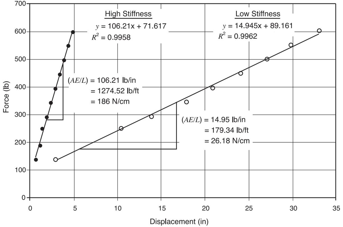
Figure 3. Load-Deflection Diagrams - Test Ropes
