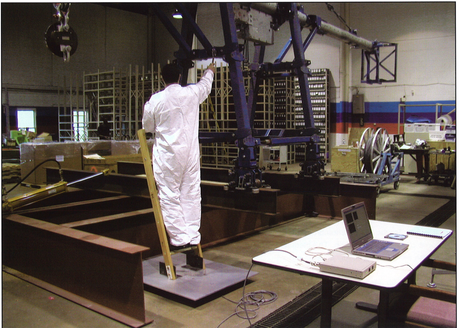
Figure 7- Force Plate Study - Side Loading of A-Frame Ladders
