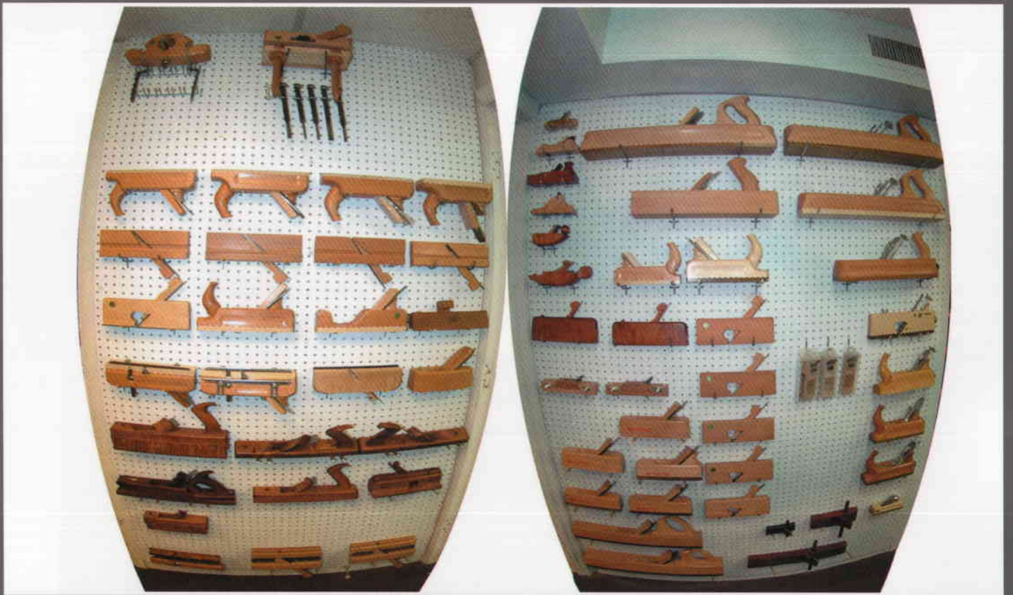
Figure 16 - Wood Plane Collection reflects soles with many complex shapes. Metal Frogs are found on the right; the other blades are held with wood wedges.
