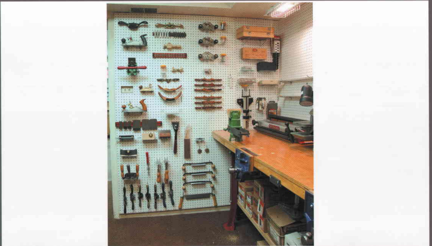
Figure 19 - Scrapers, Hand Routers, Spokeshaves, Scorp, Inshave, Shavehooks, and Burnishers (center) . Dovetail Jig (right).
