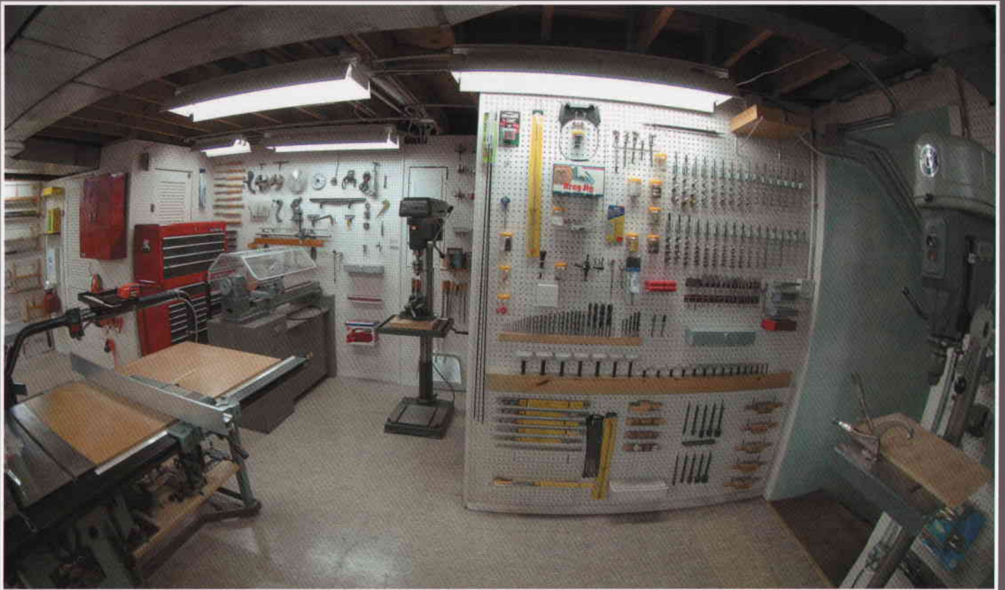
Figure 10 - Eighteen styles of Drill Bits include Spoon Bits, Gimlets, Ship Augers and Hole Saws (right). The red floor cabinet contains the only tools not on display; Wrenches, Pliers, Taps and Dies, Pincers, Sheet Metal Cutters, and Knives (left).
