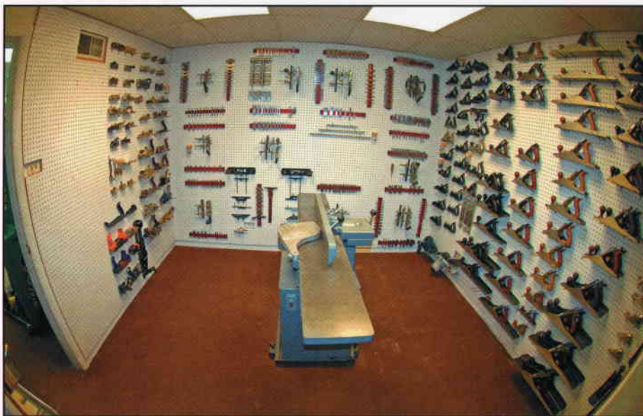
Figure 1 - It's just a plane room. The central Joiner is a stationary power tool. There are two Portable Power Planers in the lower right corner.
