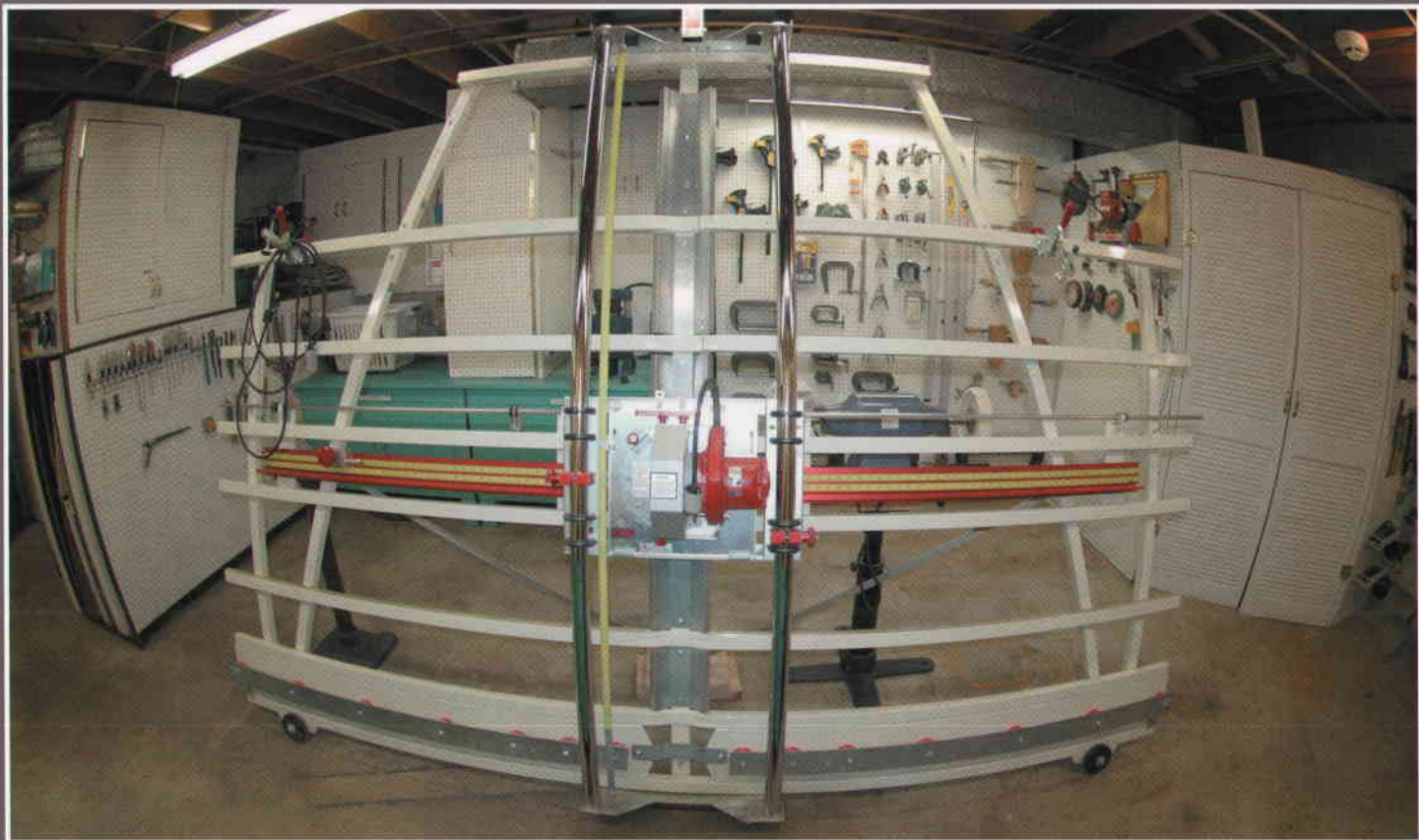
Figure 24 - Fish eye view of Panel Saw - Router. Router Attachment found at top-right of figure.
