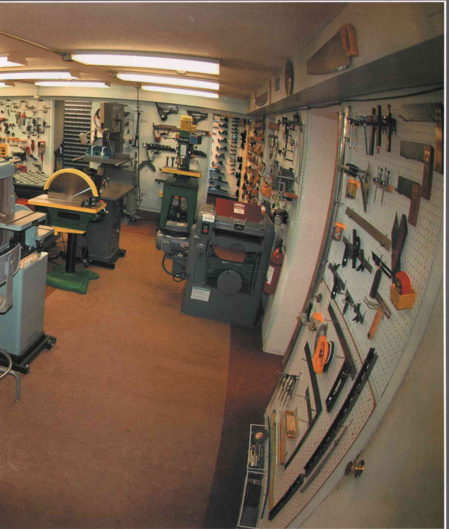
Mortiser, Oscillating Spindler Sander, and 20" Disk Sander (middle of center island). Thickness Planer (right center).
