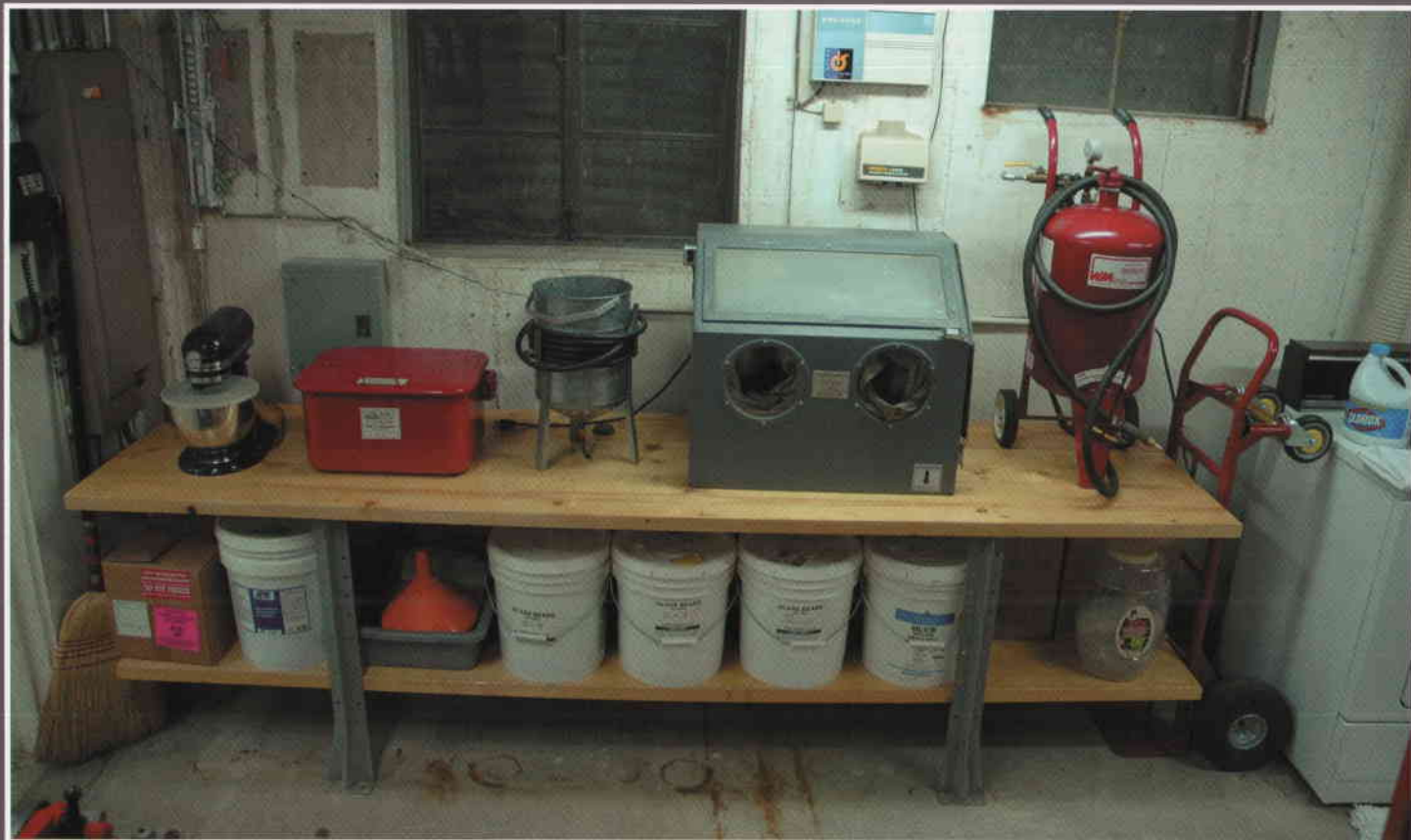
Figure 28 - Sandblasting and Cleaning Station
